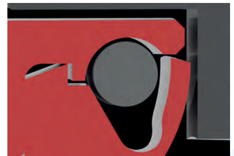
The sealing lip takes off at high speed
