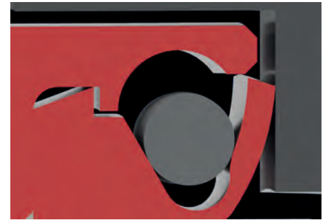
The sealing lip is in contact at low speed
