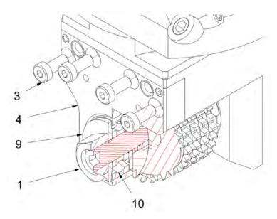
6. Now follows the fine adjustment of the finger-tight nut (Pos.1). This is conducted by adjusting the spanner nut (Pos.11) until the milling cutter has reached the required position. Finally the entire milling cutter set is tightened by the nut (Pos.1) and the spanner nut (Pos.11) is secured by the radial lock screws.
