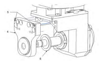
4. Mount the milling cutter (Pos.7) with the corresponding cutter spindle ring (Pos.6) onto the mandrel (Pos.8).
