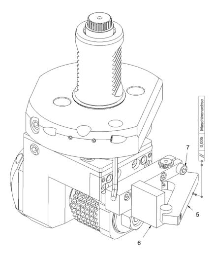
4. Tighten the hex screws (Pos.1) after reaching the requested angle. Remove the sine bar (Pos.5) before operating the machine.
