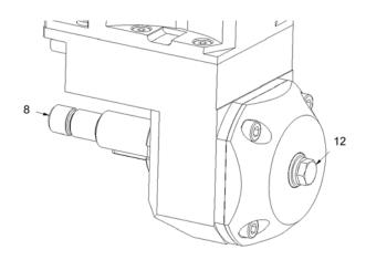
3. After the removal of the hex screw (Pos.12), pull the milling arbor forward (Pos.8) and replace it with the arbor that you want to use.
